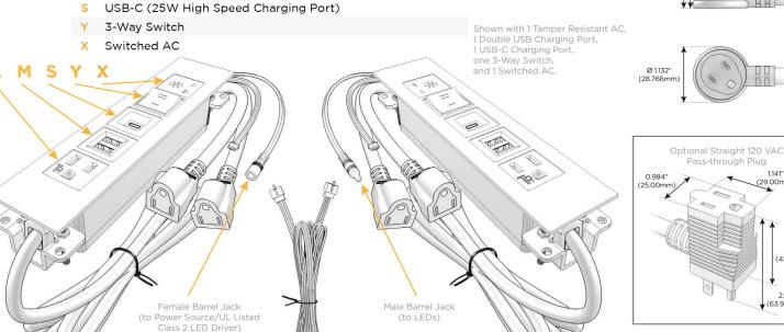
13 ft Connection Wire (connects the two outlets together)
