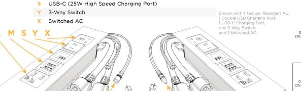
13 ft Connection Wire (connects the two outlets together)
