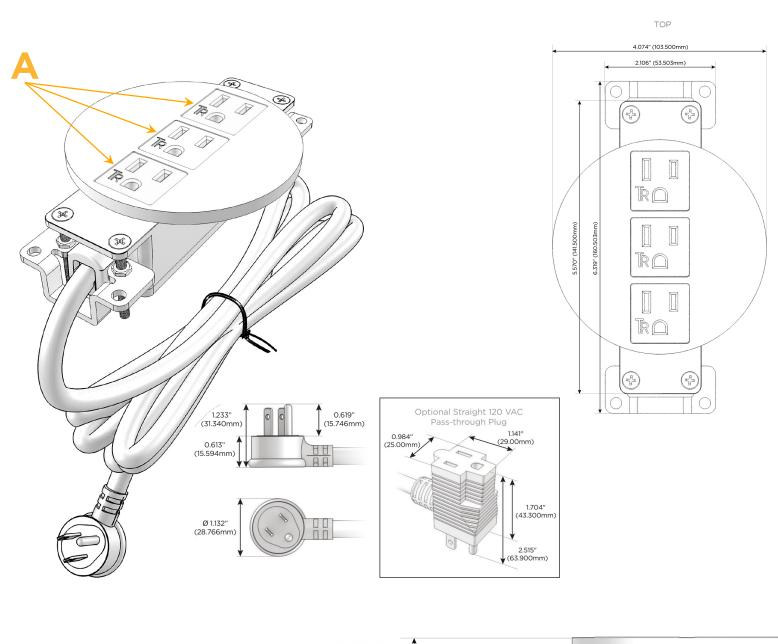
4074" (03500mm) 4074" (03500mm) END END USS" (3900mm) USS" (3000mm) USS" (3
