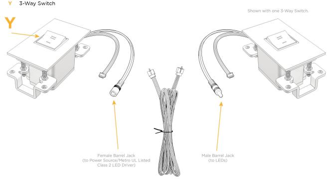
13 ft Connection Wire (connects the two outlets together)
