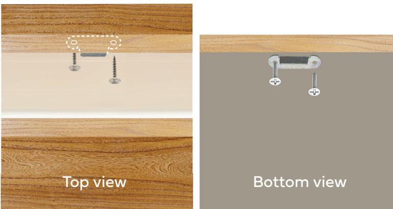
**2** Install the strike plate under the top panel as indicated in the left illustration.
